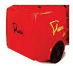
Unique smooth 'True Radius' sides allow 90° stacking with no outer turning radius.
