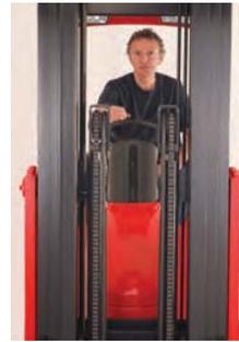
Operators have excellent forward visibility thanks to the triplex free lift mast, with its twin side mounted lift cylinders. Mast tilt means easy fork entry into pallets - even on road trailers.
